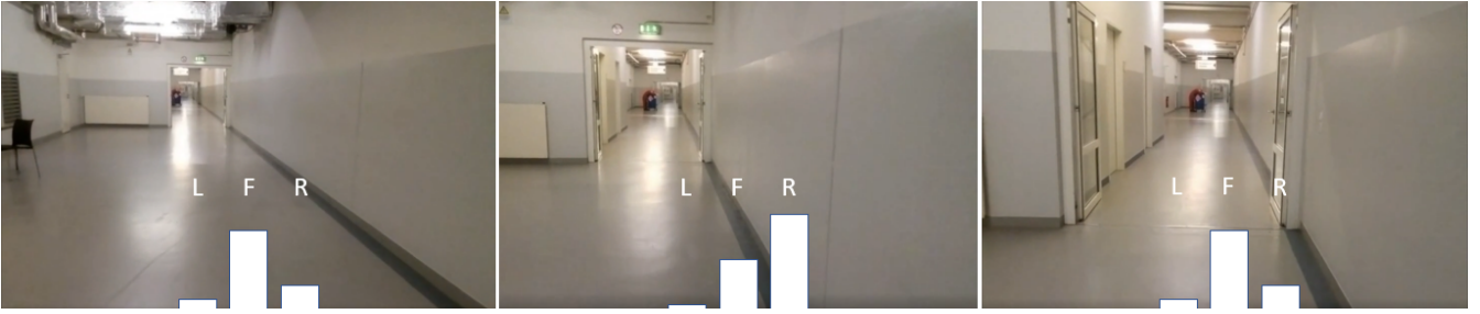
Fig. 3. Illustration of the three output classes of our neural network in different situations. The middle bar represents the velocity of the UAV directly. From the other two output values, represented by the outer bars, the turning direction is calculated by the difference between these two values.
