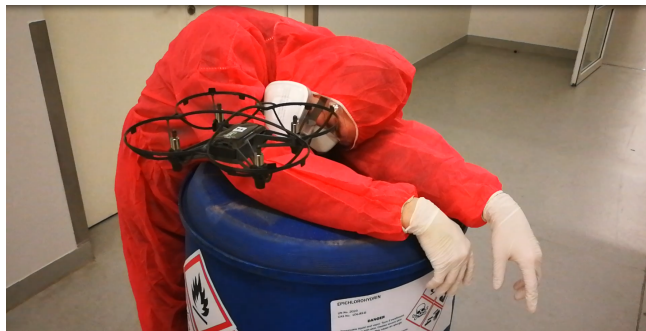
Fig. 1. Example of indoor task. A small UAV entered a building and detects an accident. The UAV is semi autonomous and remote controlled by an operator and a neural network agent (assisted autonomy). The camera images are sent to the outside operator and the AI agent. The images are processed outside and control commands are sent back to the UAV. A stable radio link connection is necessary.
