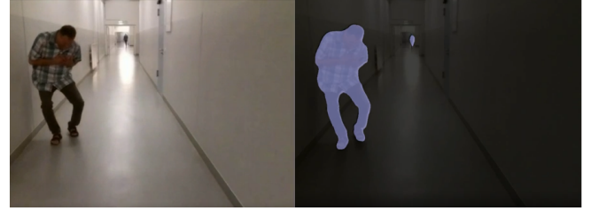
Fig. 4. Semantic segmentation of a person in acute danger in realtime using a lightweight RefineNet.
