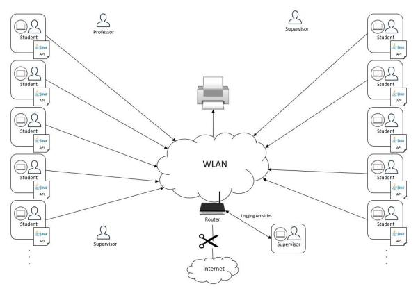
Figure 1. Technical setup for our programming exams on campus.
